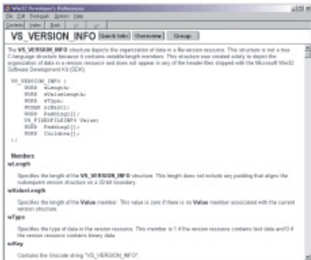
➤ Figure 2: The Microsoft documentation reveals that the version resource data can have a somewhat baroque format. Fortunately, the Delphi IDE generates a straightforward variation of this data format.
